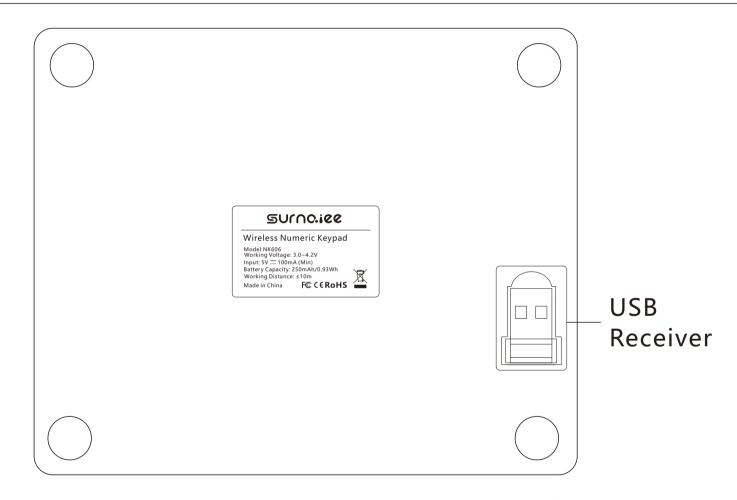
1. Take out the USB receiver on the back of the numeric keypad.
