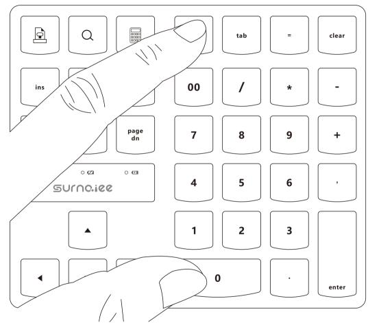
3. Press the "esc" and "0" keys at the same time and do not let go (press the "esc" key first, then press the "0" key).
