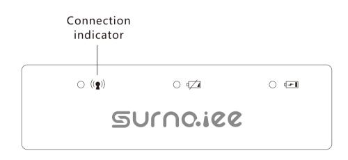
5. When the green connection indicator light on the numeric keypad stops flashing, let go of your hand, and the numeric keypad is successfully paired with the USB receiver.
