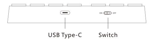
3. Turn on the switch, the connection indicator lights up for 3 seconds and then goes out, and the numeric keypad starts to work.
